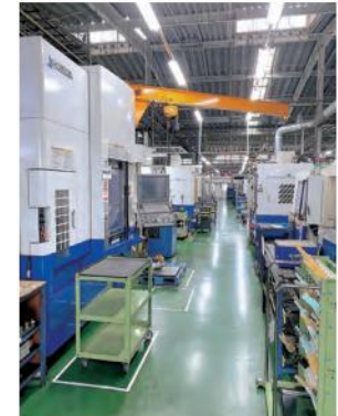
Small batch production line for torque converters
